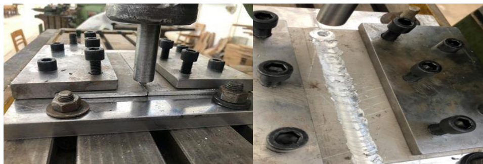
Figure.12. experimental test for welding process with a rotating speed of 315rpm and a traverse speed of 60mm/min
