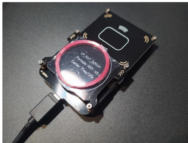
Fig.2: Image of Proxmark 3 Easy.
