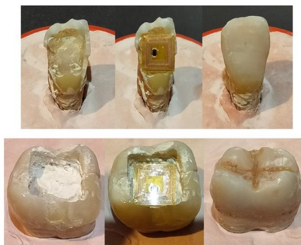
Fig.3: Canine and molar where the RFID tag has been embedded and covered with composite.
