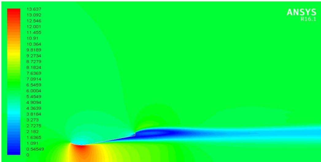
**Figure 10.** shows the velocity contour of the back flange ( $h_1 = 0.075 \cdot D = 4.5$  cm).
