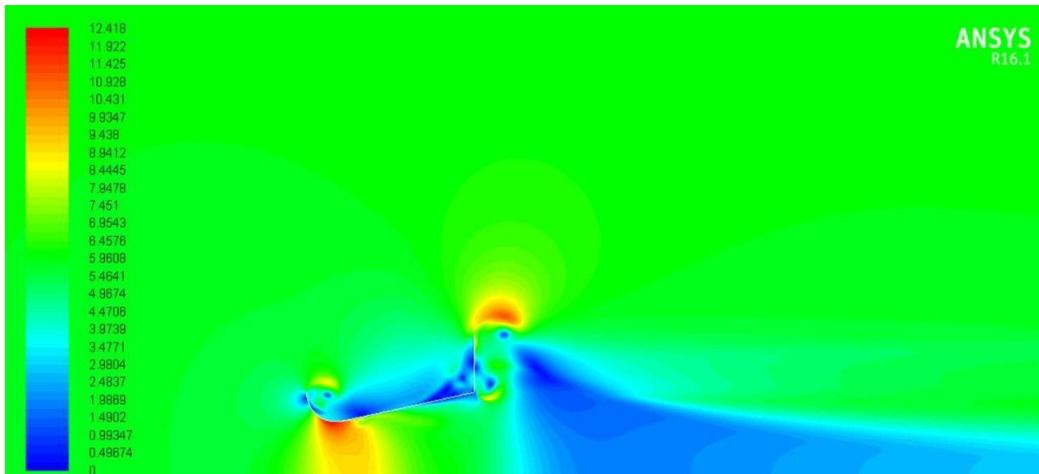
**Figure 6.** Shows the velocity contour of the entry flange radius  $R_1 = \frac{1}{4} D = 15\text{cm}$ .
