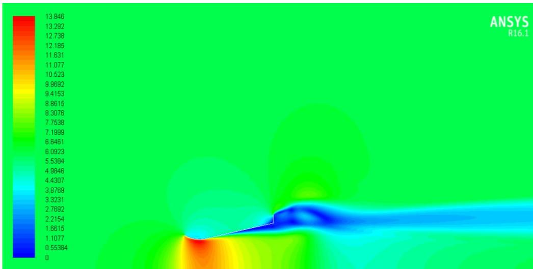
**Figure 11.** shows the velocity contour of the back flange ( $h_2 = 0.125 \cdot D = 7.5$ cm).
