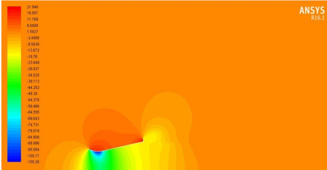
**Figure 14.** shows the pressure contour of the back flange ( $h_1 = 0.075.D = 4.5\text{cm}$ ).
