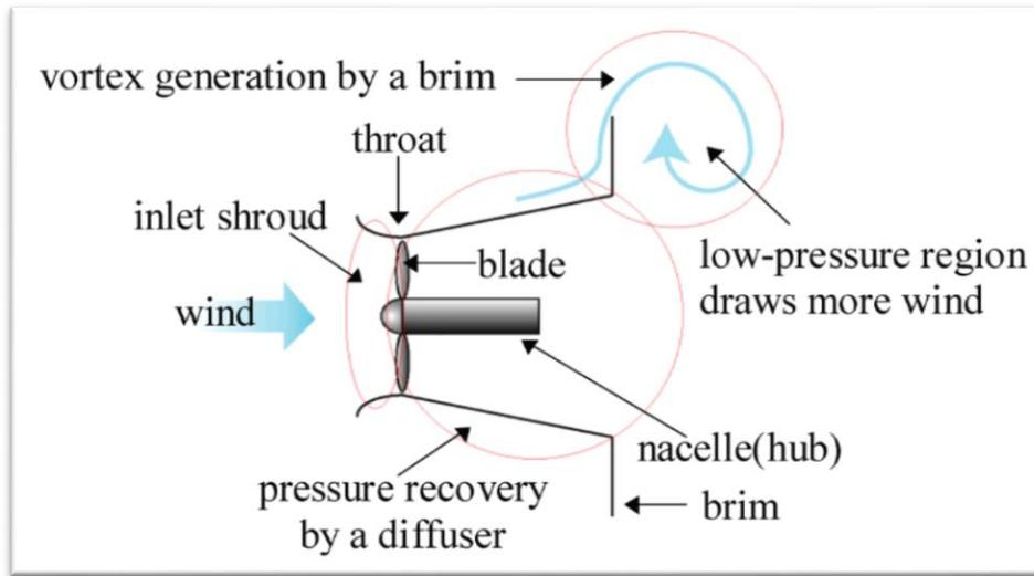
**Figure 1.** Flow around a wind turbine with brimmed diffuser.
