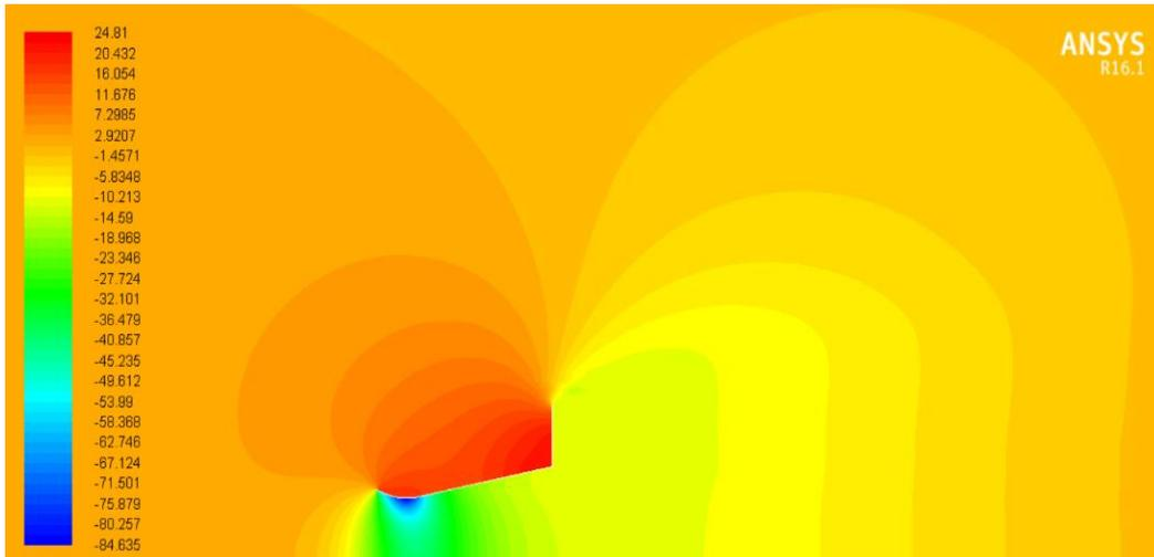
**Figure 16.** shows the pressure contour of the back flange ( $h_5 = 0.5 \cdot D = 30\text{cm}$ ).
