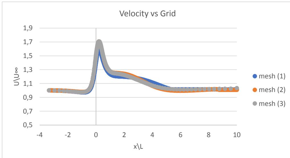
**Figure 5.** shows a comparison of flow velocity between the three meshes.
