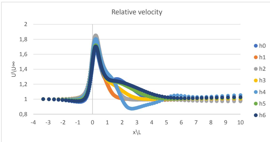
**Figure13.** relative velocity of the flow versus relative diffuser axis for the seven heights of the back flange.
