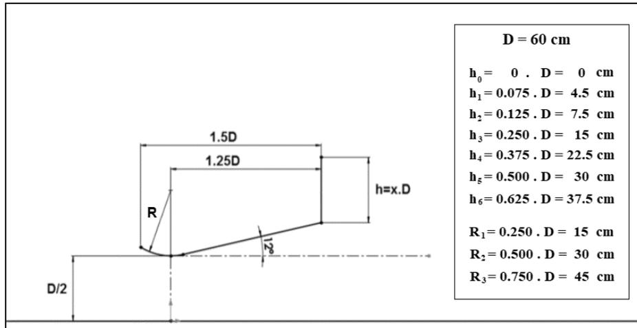
Figure 2. the geometry of the half-shroud.
