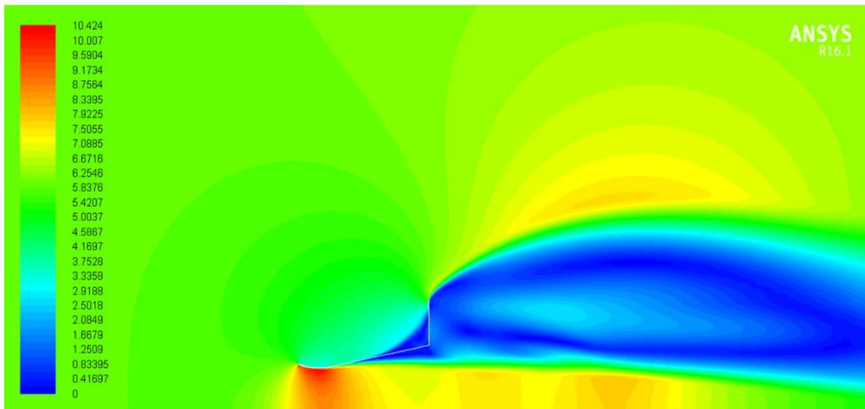
**Figure 8.** Shows the velocity contour of the entry flange radius  $R_3 = \frac{3}{4} D = 45\text{ cm}$ .
