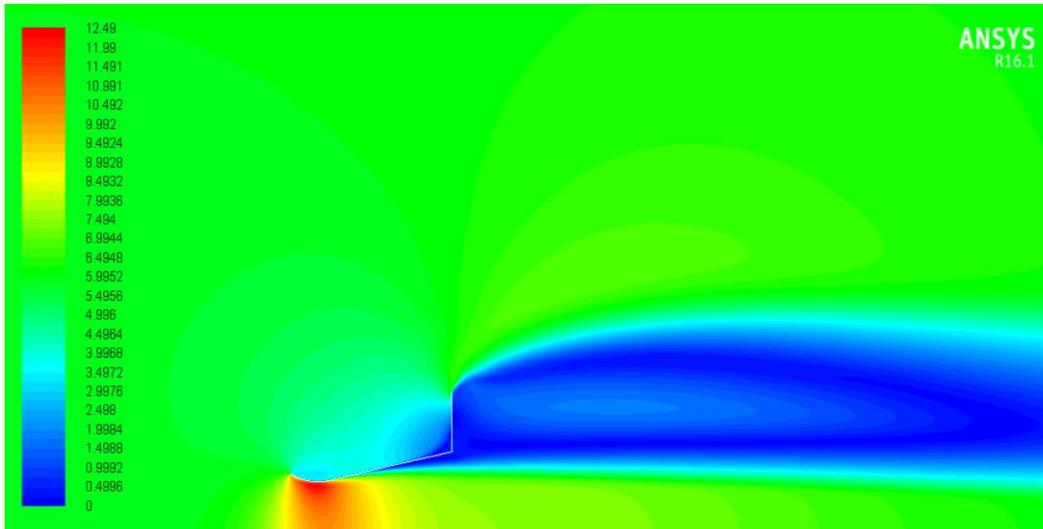
**Figure 12.** shows the velocity contour of the back flange ( $h_5 = 0.5 * D = 30$  cm).
