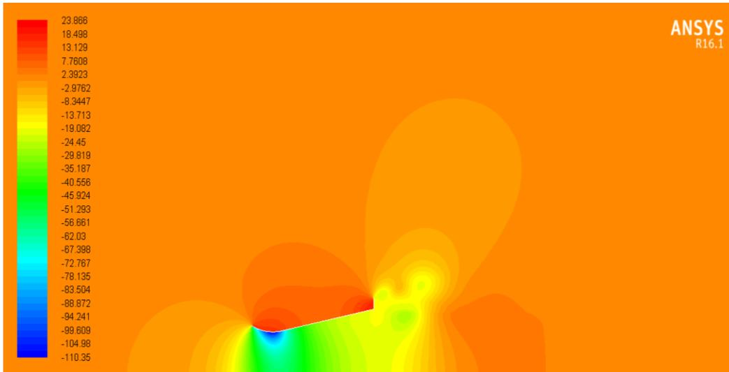
**Figure 15.** shows the pressure contour of the back flange ( $h_2 = 0.125.D = 7.5\text{cm}$ ).
