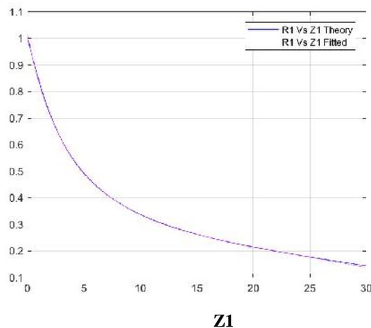
**Figure.7: Comparison of Theoretical and fitted curves for selected parameters plotted as Non-dimensional radius of the jet versus the non-dimensional distance between source and collector**
