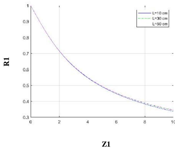
**Figure.3: Influence of spinning distance on the jet profile plotted as Non-dimensional radius of the jet versus the non-dimensional distance between source and collector**
