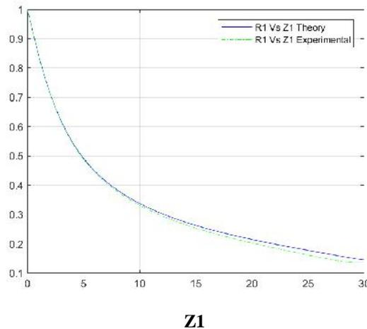
**Figure.8: Comparison of Theoretical and Experimental curves for the above selected parameters plotted as Non-dimensional radius of the jet versus the non-dimensional distance between source and collector**
