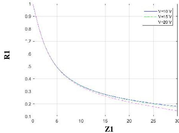
Figure.4: Influence of voltage on the jet profile plotted as Non-dimensional radius of the jet versus the non-dimensional distance between source and collector
