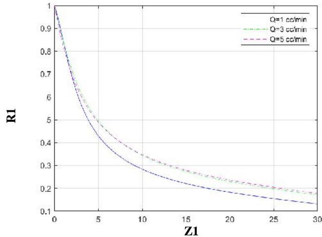
**Figure.6: Influence of flow rate on the jet profile plotted as Non-dimensional radius of the jet versus the non-dimensional distance between source and collector**
