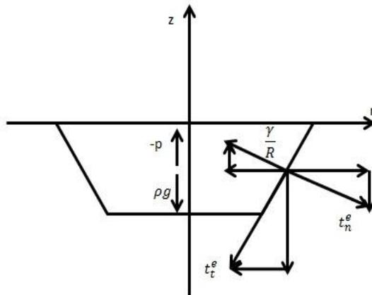
**Figure.2: Force components acting on a finiteelement of the jet**
