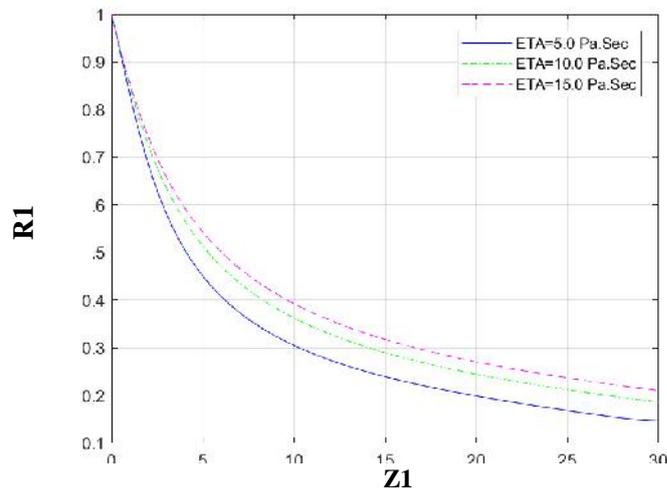
Figure.5: Influence of viscosity on the jet profile plotted as Non-dimensional radius of the jet versus the non-dimensional distance between source and collector
