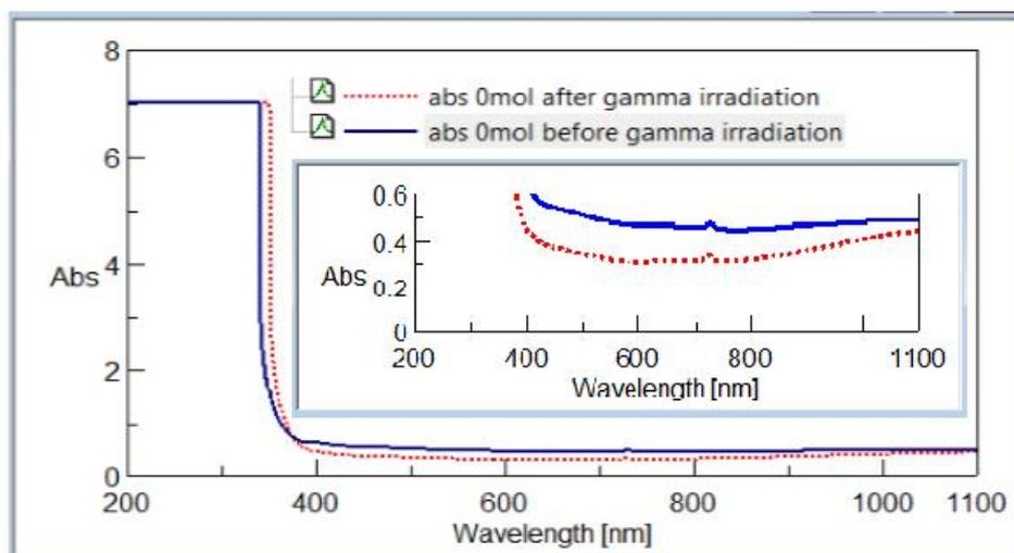
**Figure 2.** UV-visible absorption spectra of undoped(ZAP) glass before and after gamma irradiation
