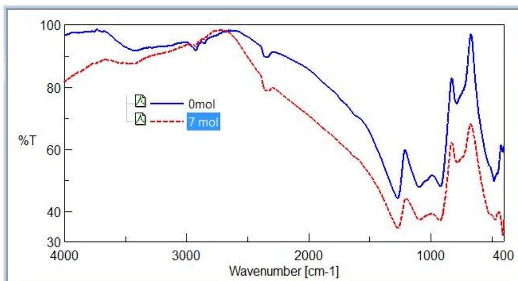
**Figure 4.** FTIR infrared transmittance spectra of undoped and  $\text{CeO}_2$ -doped (ZAP) glass before gamma irradiation
