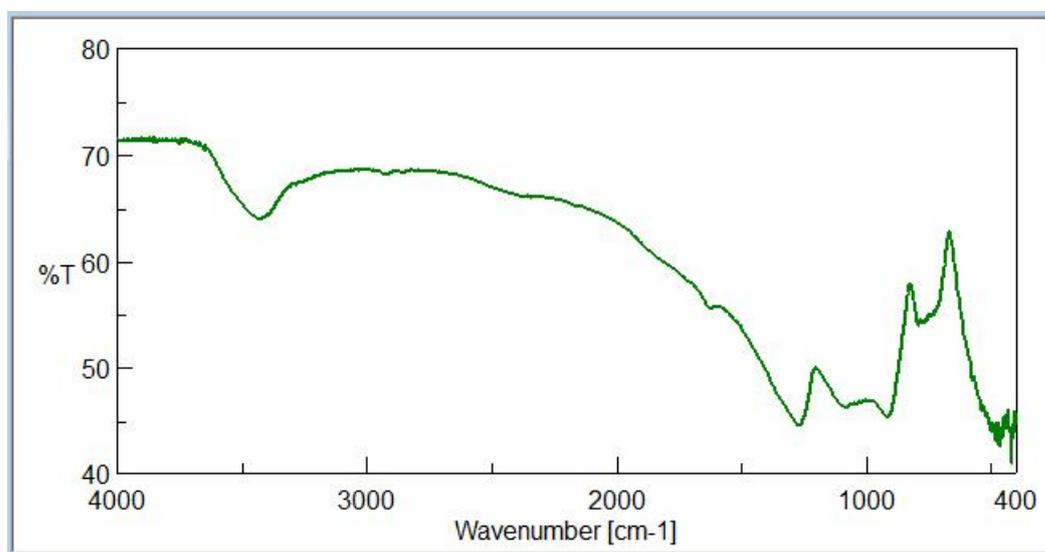
**Figure 5.** FTIR infrared transmittance spectra of CeO<sub>2</sub>-doped zinc – aluminum phosphate glass after gamma irradiation
