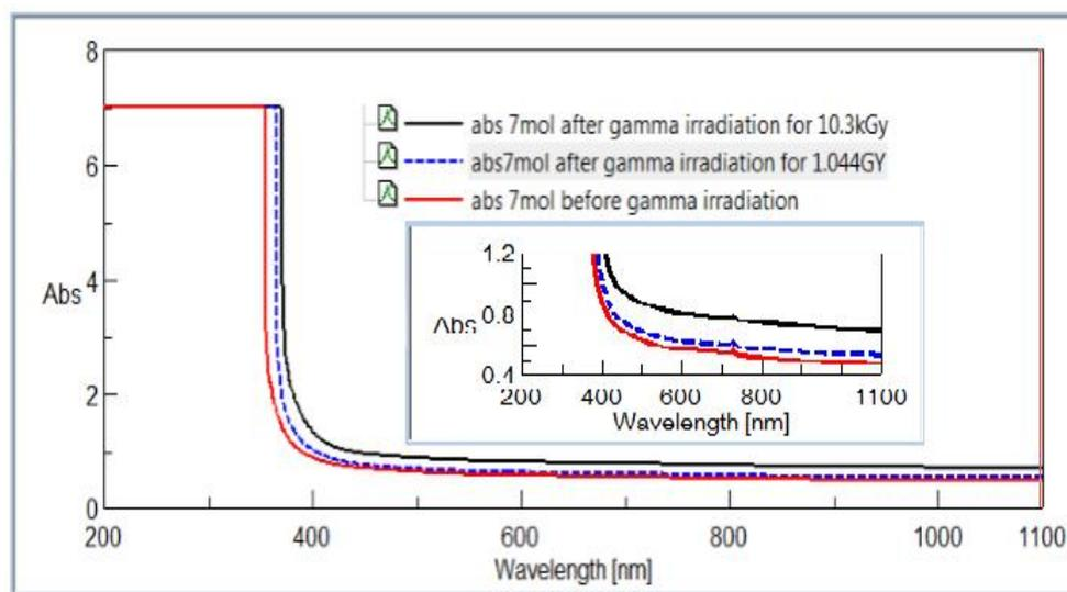
**Figure 3.** UV-visible absorption spectra of 7% CeO<sub>2</sub>-doped (ZAP) glass before and after gamma irradiation
