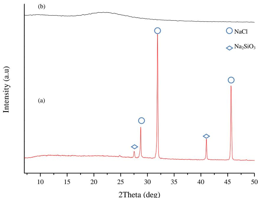
**Fig. 2.** XRD patterns of silica (a) unwashed and (b) washed.
