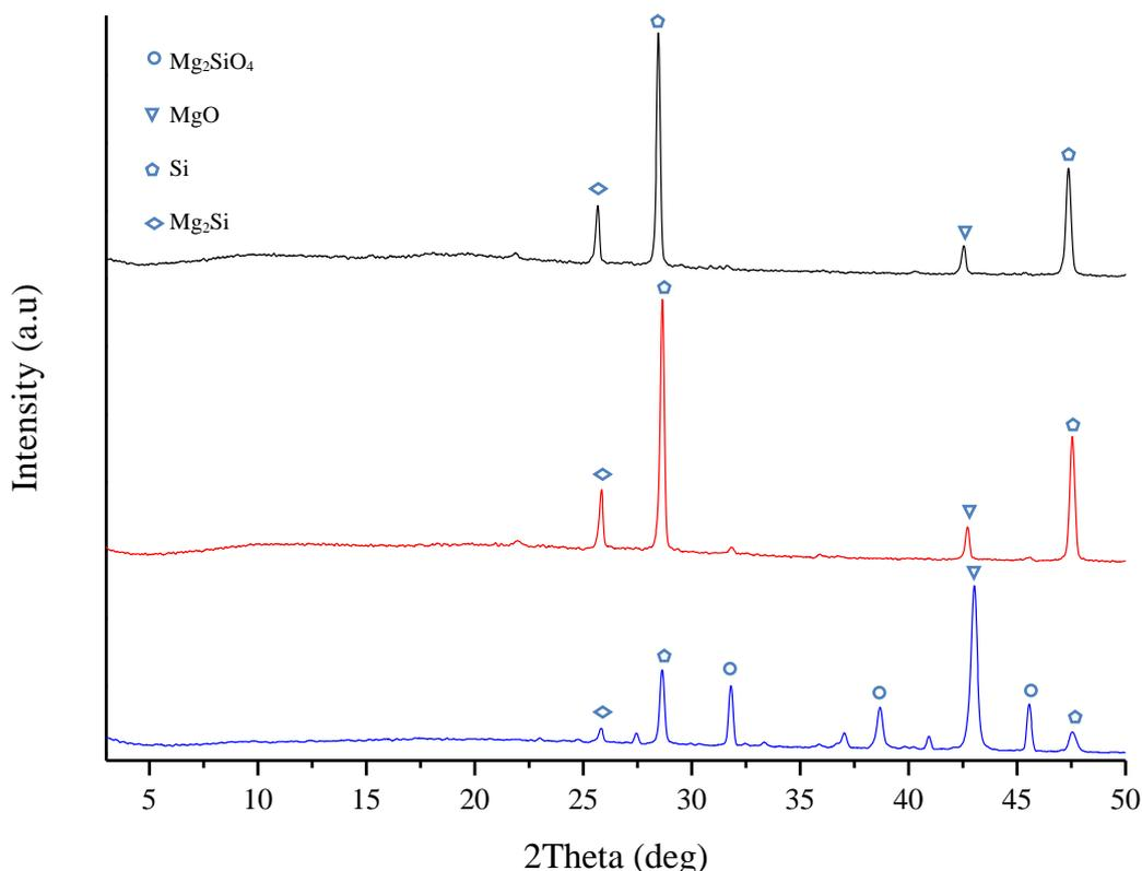
Fig. 3. XRD patterns of (a) Si-unleach, (b) Si-leach 1, and (c) Si-leach 2
