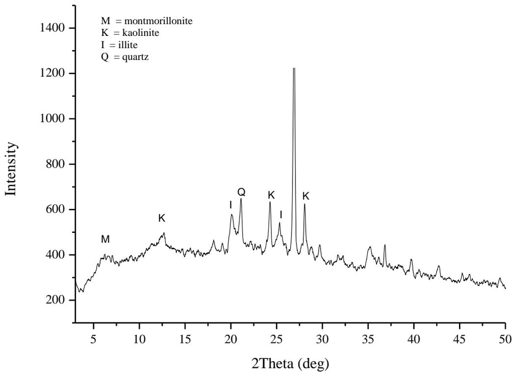
**Fig. 1.** X-ray diffratogram of the Lapindo mud
